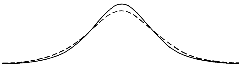
FIGURE 14. Free-surface profile —, initial condition of a solitary wave of translation of height 0.2134; - - -, instantaneous profile after nine reflections.
